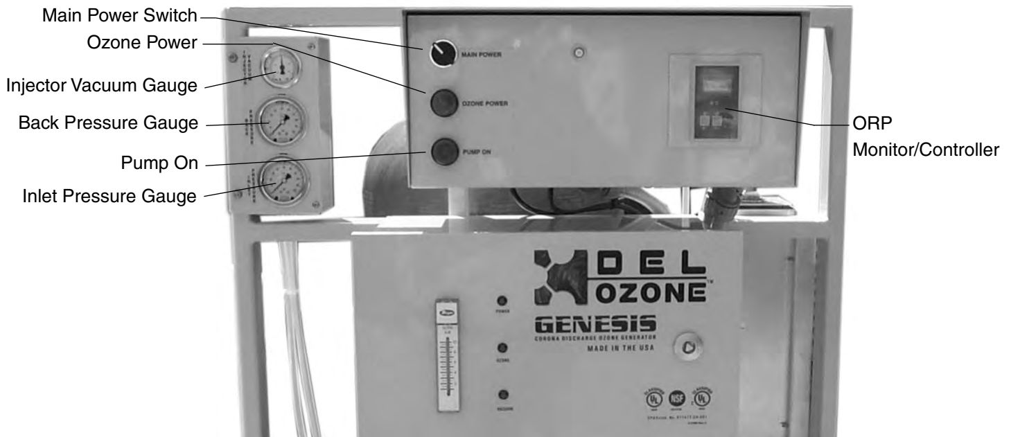
Figure 2: CPS-8000 Control Panel
